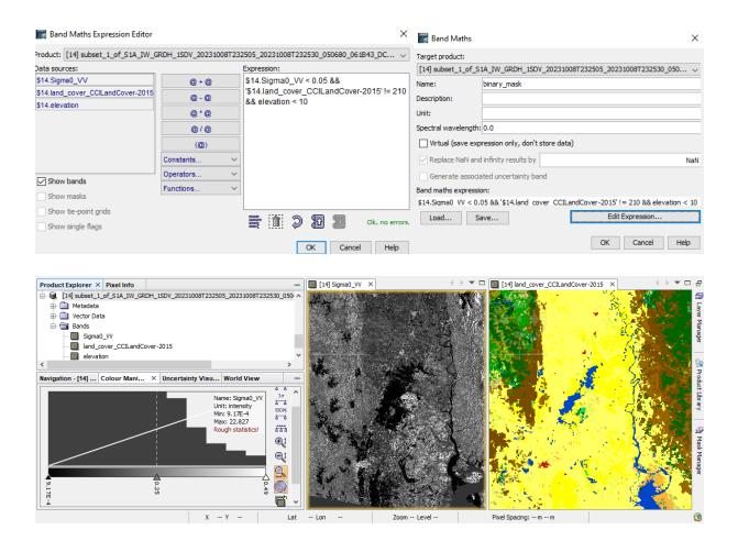
Repeat the process for the second Sentinel product. Display the two masks to check they have been generated correctly. Our output flooding binary band should look like this (For September  $26^{th}$  – start of flodding and October  $10^{th}$  – peak of flooding):
