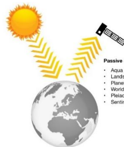
PASSIVE Earth Observation Satellites Passive satellites detect radiation reflected off the Earth's surface, such as visible light and infrared. In general, passive satellites are not able to work through clouds.
