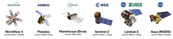
PASSIVE Earth Observation Satellites Passive satellites detect radiation reflected off the Earth's surface, such as visible light and infrared. In general, passive satellites are not able to work through clouds.
