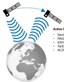
ACTIVE Earth Observation Satellites Active satellites transmit energy towards the Earth and measure the returned signal which provides information about the Earth's surface. In general, active satellites can see through clouds.
