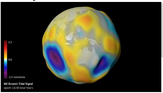
The magnetic tidal signal measured by Swarm is important for ocean and climate modelling, and is used to determine the electrical properties of the Earth's lithosphere and upper mantle.
