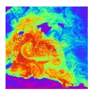
In this night-time image of SST from AATSR, the coldest areas - which include all the land - are shown in purple and blue, whilst yellow and orange are used to represent successively warmer temperatures over a total range of 280-295 K. Credit: RAL
