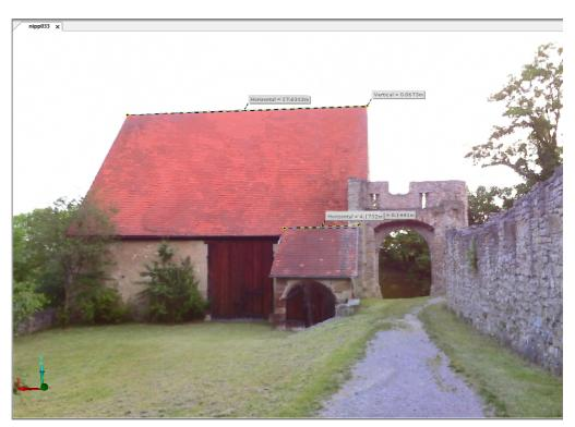
Figure 10-2 Point-to-point measurement
