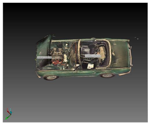
Figure 10-21 Example: Complete point cloud
