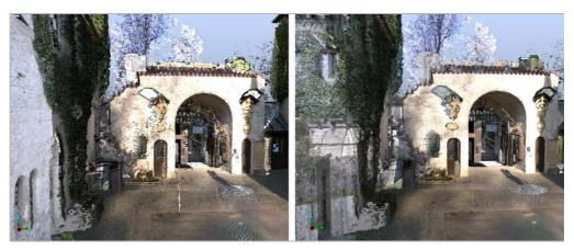
Figure 5-4 Supersampling turned off (left) and turned on (right)
