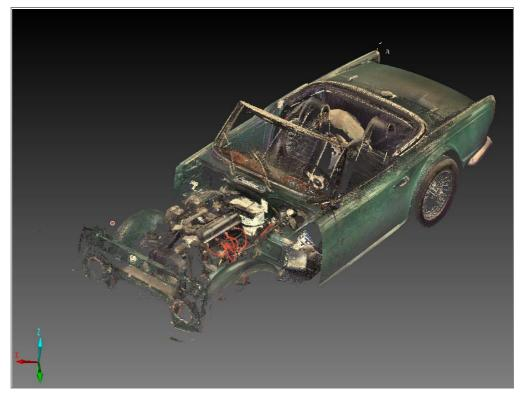
Figure 10-25 Example: Result with hidden Clipping Boxes
