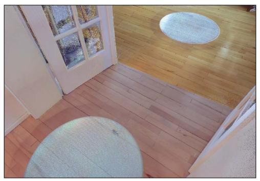
Figure 10-3 Inconsistent color of a floor due to scans taken under varying lighting conditions.
