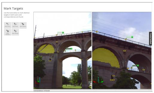
Figure 9-5 Split View with detected correspondences
