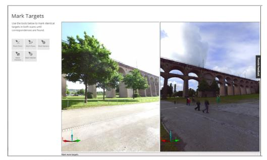
Figure 9-4 Manual Registration task, second step: select targets
