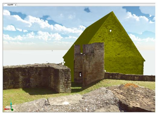
Figure 10-4 Scan points of a house, marked with the Polygon selection
