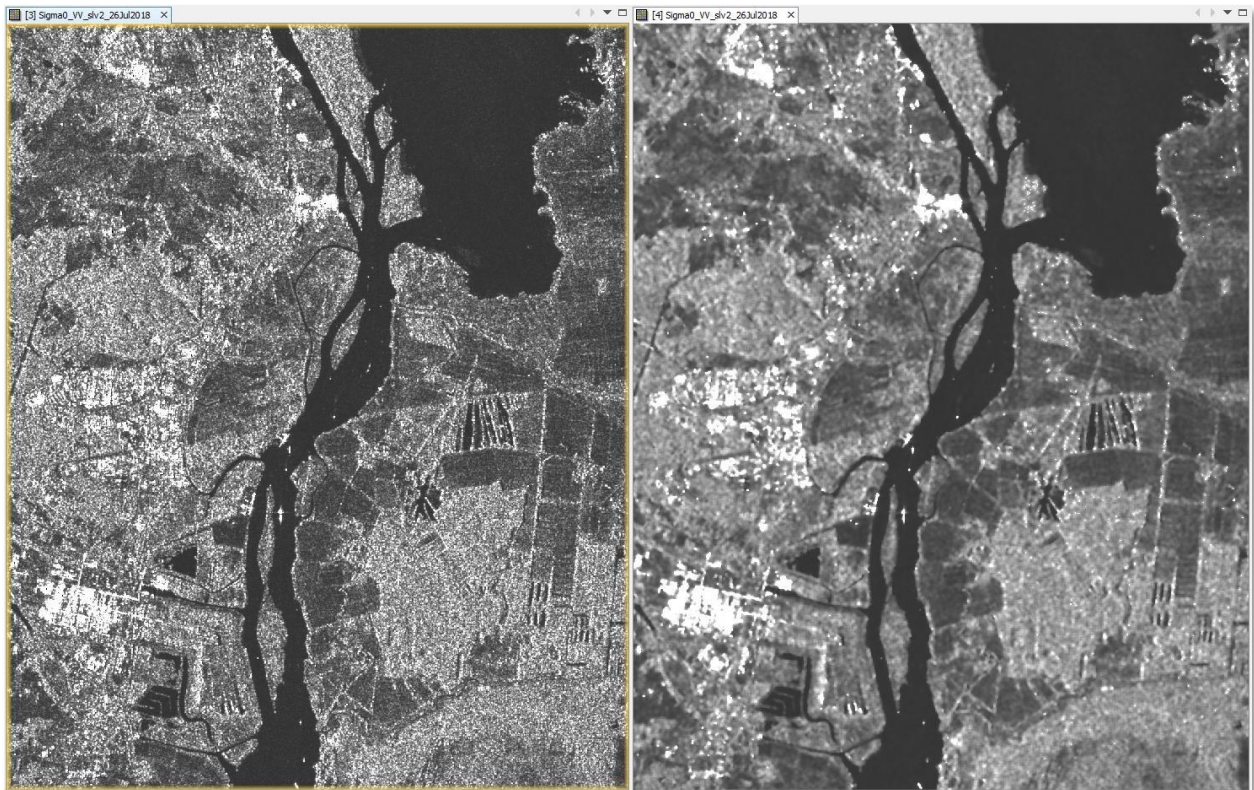
Figure 14: Sigma0 VV before (left) and after (right) application of a speckle filter
