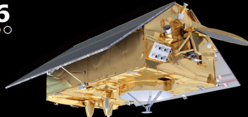
Sentinel 6 - Jason-CS (A/B) – Low inclination Altimetry Sea-level, wave height and marine wind speed
