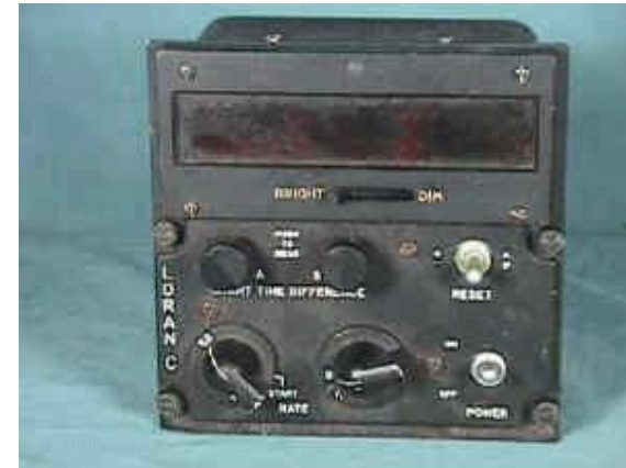
C-6430/ARN-78 Loran C Aircraft Control Box.
