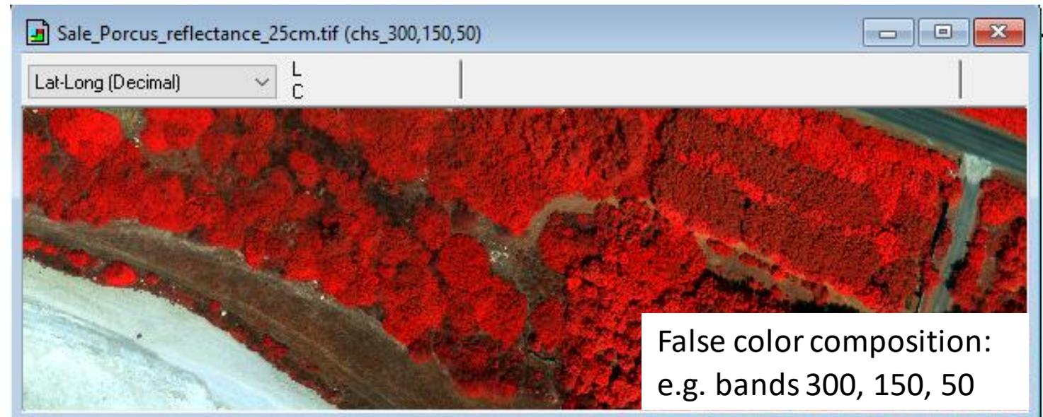
An example of displaying the false color composition using data from the HS scanner AISA KESTREL and the corresponding RGB bands of the scanner.
