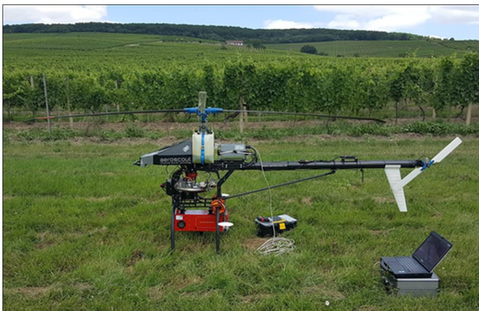
Fig. 2. The Scout B1-100 remotely piloted helicopter powered by a gasoline two-stroke engine with the hyperspectral payload in the red box coupled with a dual GPS antenna during data download in the vineyard of “Hon Makovisko”, Malá Trňa owned by Ostrožovič s.r.o.,
