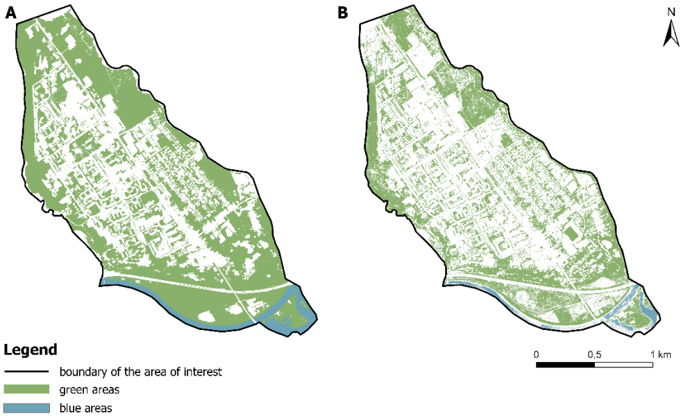
Fig. 4. Green and blue areas identified from orthophoto mosaic using: A – using deep learning method, B – NDVI and NDWI index
