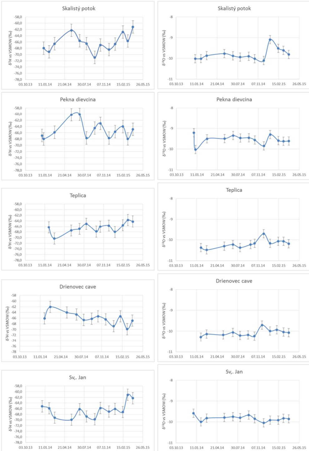
**Fig. 9.** Hydrogen (left) and oxygen (right) isotope ratio time series of the spring water samples
