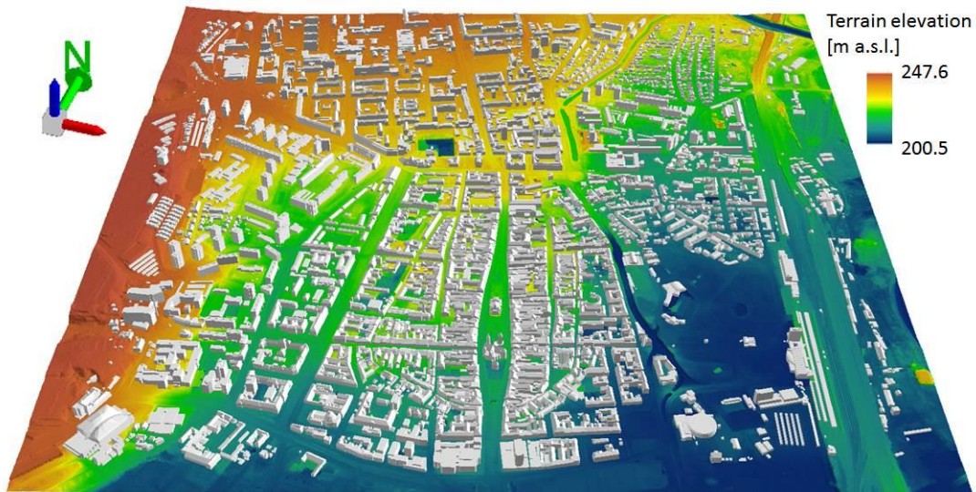
Figure 3: Perspective 3D view of the entire study area (cyan outline in Fig. 1) for which the 3D city model was generated. 3D buildings are displayed on a digital terrain model in the ArcScene software by ESRI.
