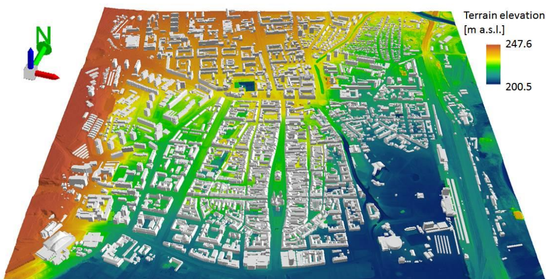
Figure 4. Perspective 3D view of the entire study area (cyan outline in Fig. 1) for which the 3D city model was generated. 3D buildings are displayed on a digital terrain model in the ArcScene software by ESRI.
