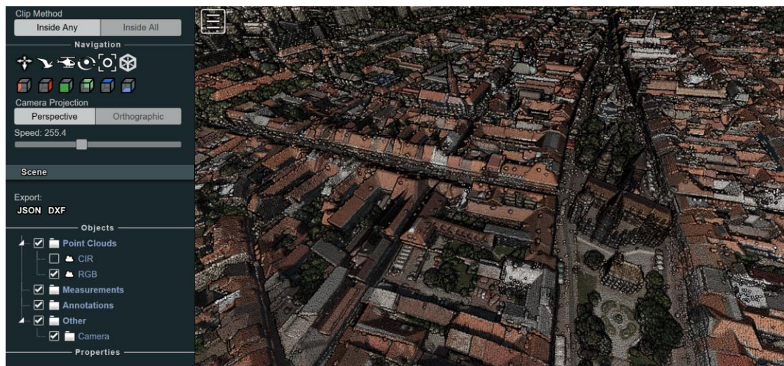
Figure 5. ALS dataset of the Košice city visualized in an interactive web interface based on the Potree renderer (Institute of Computer Graphics and Algorithms, TU Wien) and laspublish software by rapidlasso GmbH. Available at: https://esa-surge.science.upjs.sk/laspublish/ALS_Kosice.html
