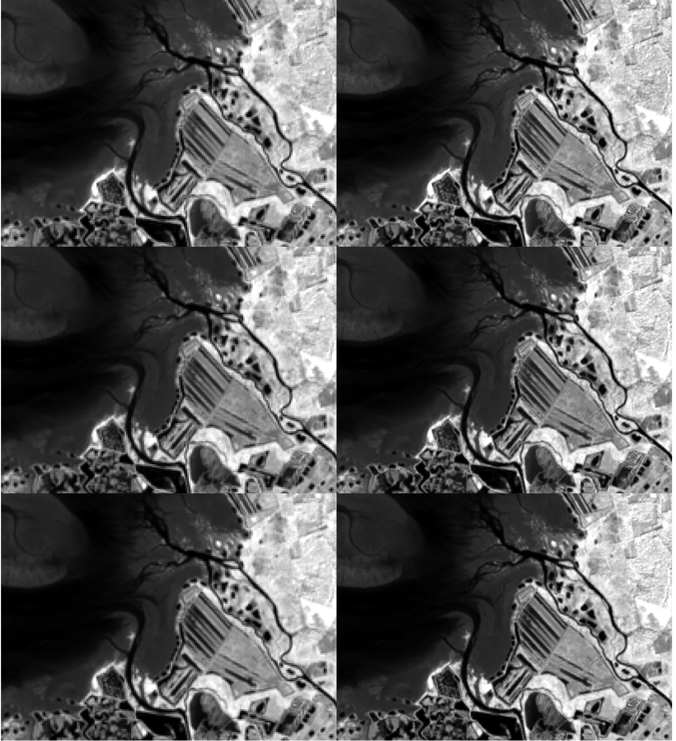
Figure 6. Coastal area (delta of the Leyre river). Top-left: Original band 6 (close infrared, 740nm, 20m/pixel). Top-right: Super-resolved band 6 at 10m/pixel. Middle-Left: Original band 7 (close infrared, 783nm, 20m/pixel). Middle-Left: Super-resolved band 7 at 10m/pixel. Bottom-left: Original band 8A (close infrared, 865nm, 20m/pixel). Bottom-right: Super-resolved band 8A at 10m/pixel.
