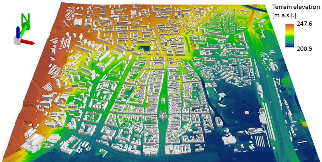
Figure 4. Perspective 3D view of the entire study area (cyan outline in Fig. 1) for which the 3D city model was generated. 3D buildings are displayed on a digital terrain model in the ArcScene software by ESRI.
