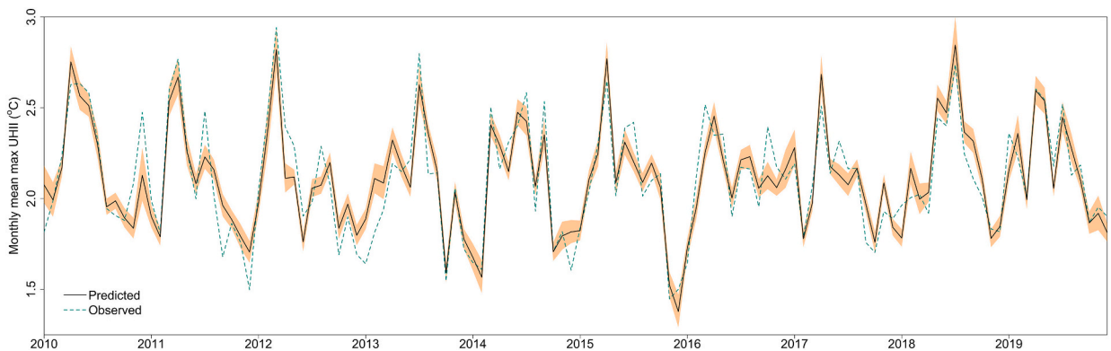
Fig. 4. GAM predicted monthly mean maximum UHII compared with observed between 2010 and 2019. The 95% confidence intervals from the GAM model are provided in orange shading.
